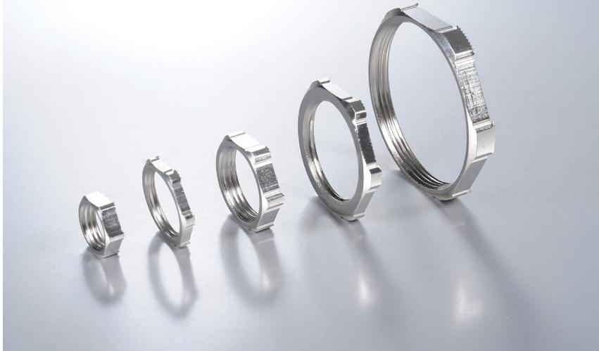
To ensure permanent bonding between the cable gland and housing in painted or coated housings, a lock nut with 6 teeth which cut into the coating automatically when tightened, thus providing equipotential bonding. Moreover, this type of attachment increases the installation's resistance to vibration.
